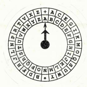
The first letter of the message is 'K'. The device is advanced tensteps clockwise, so that the shorter hand now points to 'K' in the inner circle. The longer hand points to 'S' in the outer circle. The first character of the enciphered message is therefore 'S'.
