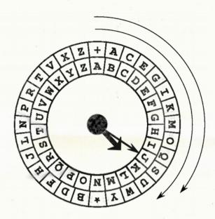
The second letter of the message is 'E', so the device is advanced clockwise (always clockwise) twenty step until the shorter hand points to 'E' in the inner circle. The longer hand advances twenty steps also, and now points to 'C' in the outer circle. The second character of the ciphertext is therefore 'C'.
