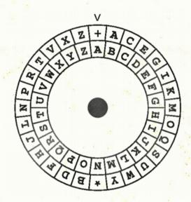
The device is aligned to its initial position. The shorter hand points to 'A' in the *butlet* inner circle, and the longer hand points to '+' in the outer circle ('+' is the first character of the key).
